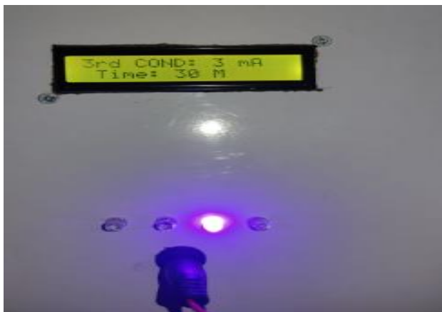
Figure 07: The result achieved at 3rd condition in which 3mA current is delivered to the patient for 30mints.
