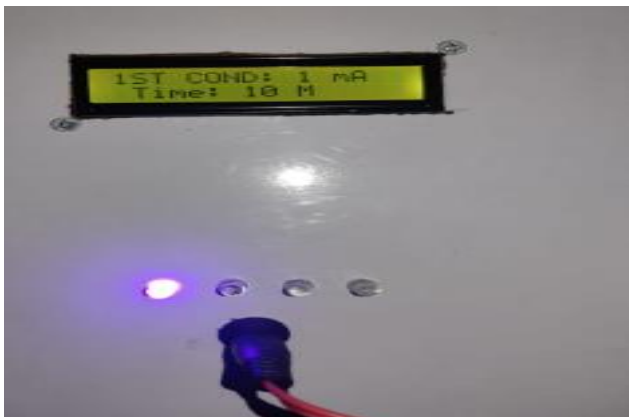
Figure 05: The result achieved at 1st condition in which 1mA current is delivered to the patient for 10mints.
