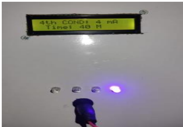
Figure 08: The result achieved at 4th condition in which 4mA current is delivered to the patient for 40mints.
