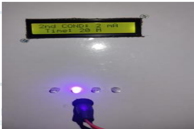
Figure 06: The result achieved at 2nd condition in which 2mA current is delivered to the patient for 20mints.
