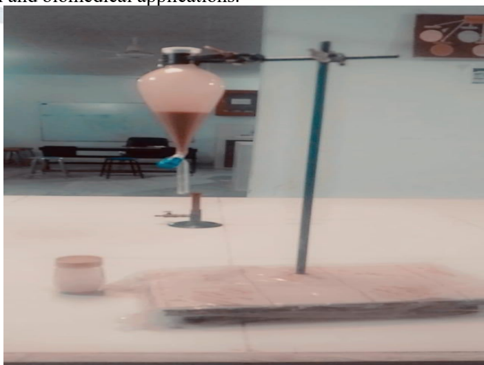
Figure 2.1: illustrates the funnel separation process employed to isolate castor oil from the aqueous mixture after the initial extraction steps.
