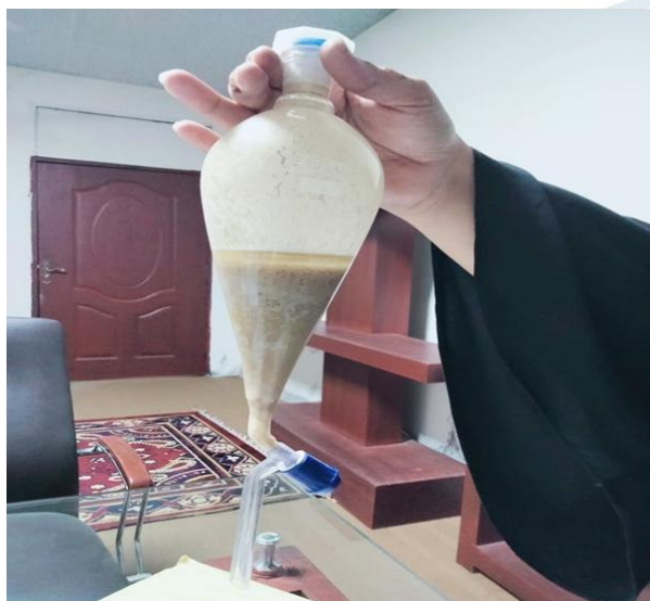
Figure 2.2: (a) illustrates the separation process of castor oil from an aqueous solution following extraction with acetone. (b) the timeline of oil yield during the extraction process is presented.
